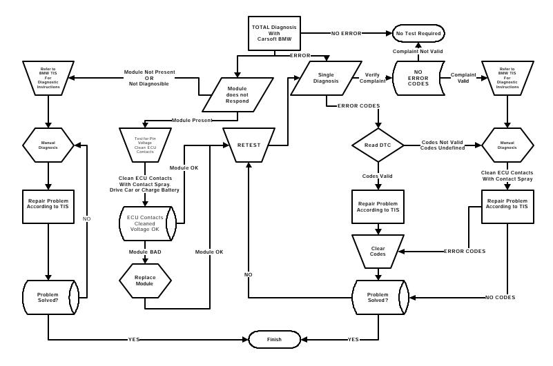
This flow chart outlines the required steps of normal diagnosis. To verify codes on new cars, LIVE DATA functions may be utilized. On older cars, manual diagnostics is required.
